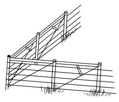
Figure 11. Double H Brace Assembly (Corner).
