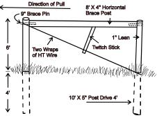
Figure 10. Single Span Brace Assembly
