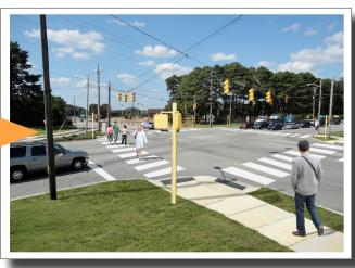
Photo visualization showing high visibility crosswalks and pedestrian activated countdown signals.
