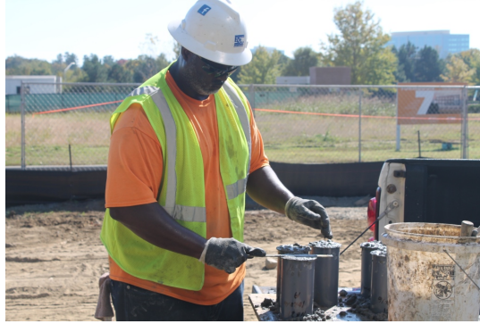
Concrete Strength Testing
