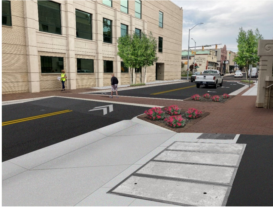
Figure 3: Proposed raised pedestrian crossing on West 5 th Street at City Hall and Municipal Building
