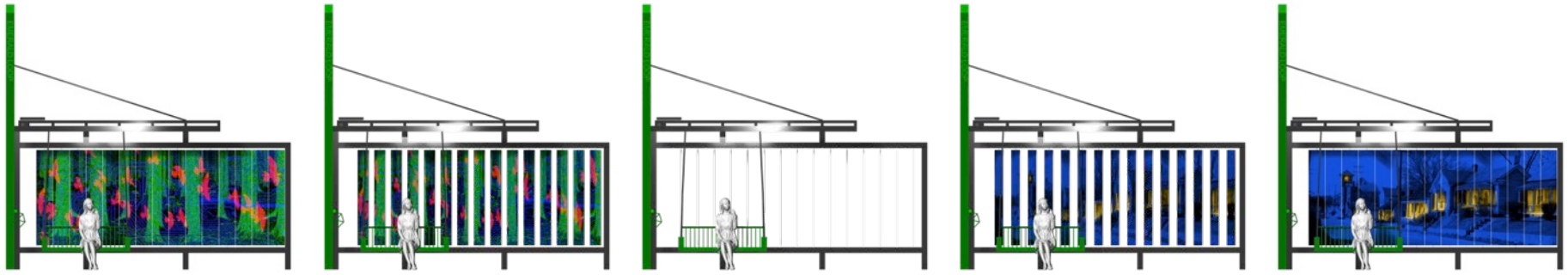
Sequence showing 180-degree rotation of fins
