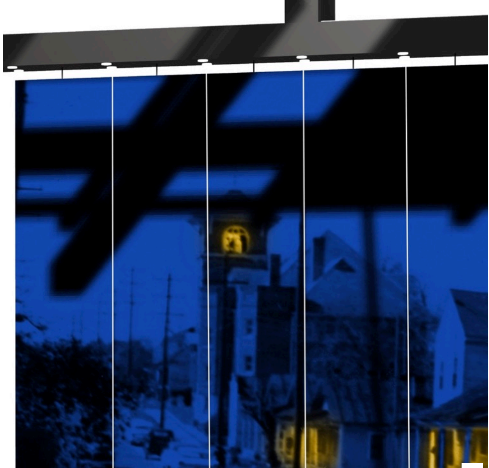
Rotating fins require two LEDs between fins, to illuminate both sides i... closed position
