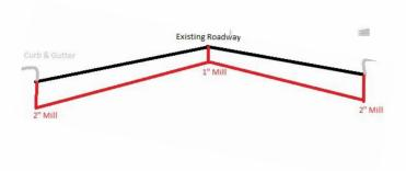
2" milling on the edges with a 1" mill in the centerline.
