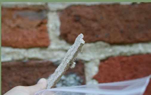
A piece of failed repointing mortar is held up to show how thinly it was applied.
