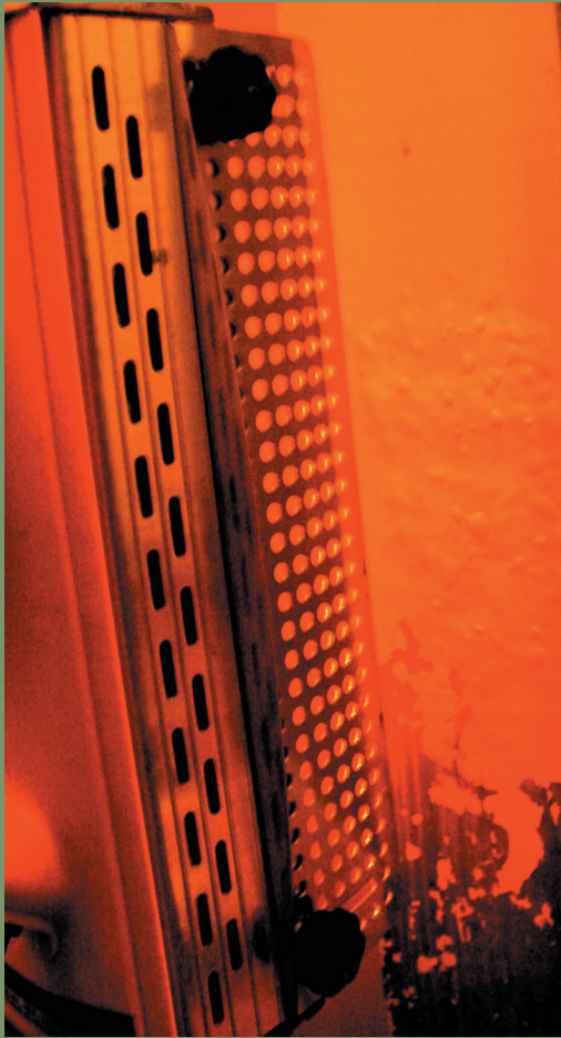
Paint quickly releases from the wood surface and bubbles under the heat of an infrared paint remover.
