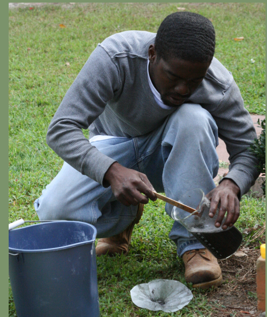
A mason demonstrates a quick field characterization of a mortar sample for Edgecombe Community College Preservation Trades students. By dissolving the binder of the mortar, the aggregate particle size, distribution and color can be examined as well as any additives that remain.
