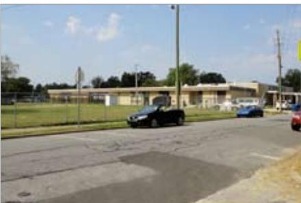
*Fleming School crosswalk - lacks curb ramps, in-roadway signage, high-visibility marked crosswalk, and bulbouts*
