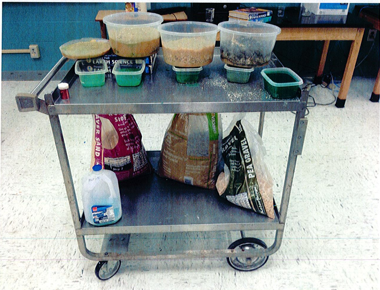
Figure 2. Simulated BMPs from left to right: greenroof, bioretention with internal water storage, bioretention, and permeable pavement. Containers below BMPs contain treated stormwater. The container on the far right contains simulated stormwater. Below are materials used in making simulated BMP from left to right: paver sand, large gravel, and pea gravel. A 1-gallon jug with a perforated lid was used to sprinkle stormwater on BMPs.
